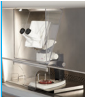
This LabGard BSC was fitted with a microscope viewing window to accommodate workflow specializing in human cell tissue research.
